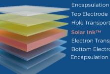
Hole Transport Layer Solar Ink™ Electron Transport Layer Bottom Electrode Encapsulation
