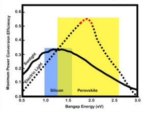
Theoretically, the best absorber materials for indoor application should have a band gap between 1.8 to 2.0 eV. That's why silicon, with a bandgap between 1.1 to 1.6 ev shows poor performance for indoor light.
